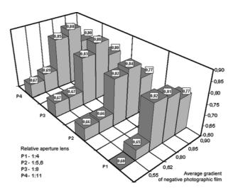
Figure 5. Relation of general gradient of the tone -reproduction curve to the gradient in half-tones versus values of the relative aperture lens and average gradient of negative photographic film
